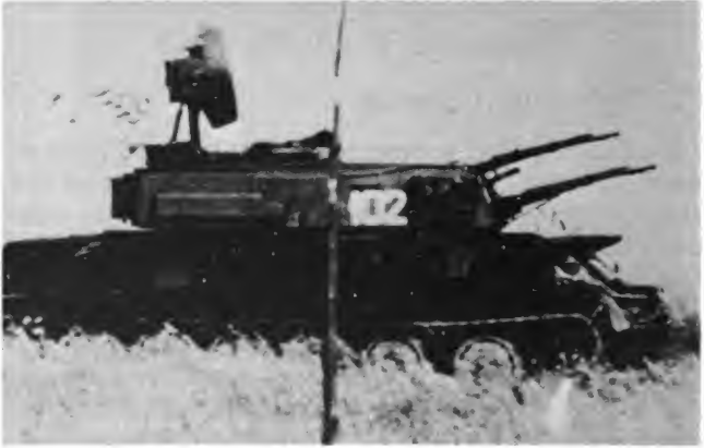
Figure 5-8 . Air and tank defense. Tracked anti-aircraft vehicles, such as the 23-mm ZSU-23-4 (above), provide mobile air defense for armored striking forces. Motorized rifle squads are equipped with RPG-7 anti-tank grenade launchers (below).
